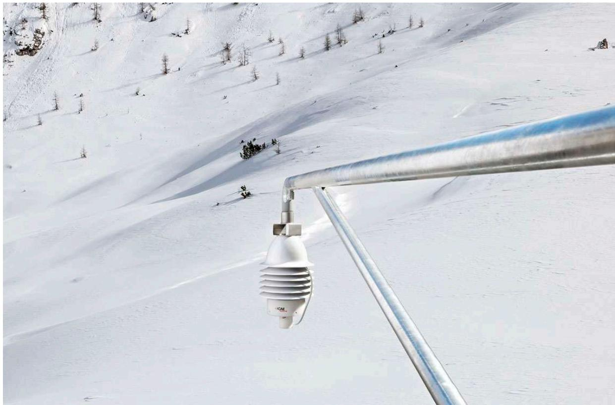
The sensor has a real time clock and a permanent storage memory and communicates with other modules via: Caenet bus, standard SDI-12 protocol on RS485 and 4-20 mA analogue output. This allows interfacing with any datalogger.
